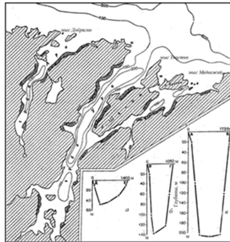
Fig. 2. Map-scheme of big fjords along Murman's coast of the Barentz Sea. Fragments a , b and c are integral transversal profiles across of fjords: a and b – Ara-guba fjord; c – Ura-guba fjord. Vertical axis is depth (meters); horizontal axis is width of fjord, in meters. Dark contour of the shore as a sites of abrasive-denudate cliffs (according by P. A. Kaplin [8])
